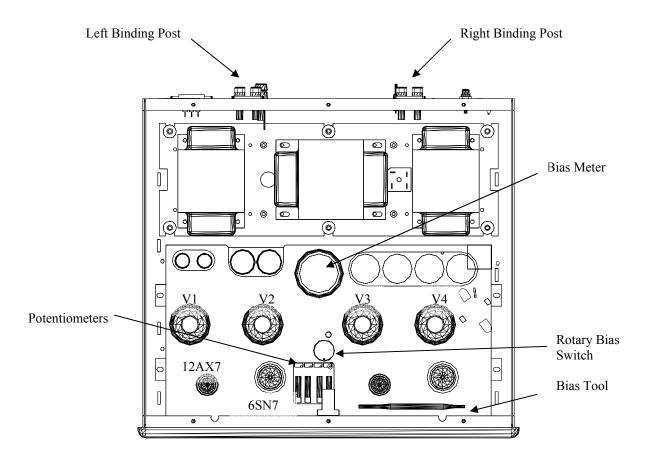
Figure 1 Tube and Deck Layout
