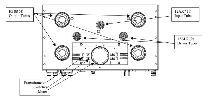
Figure 3. Bias switches and potentiometers
